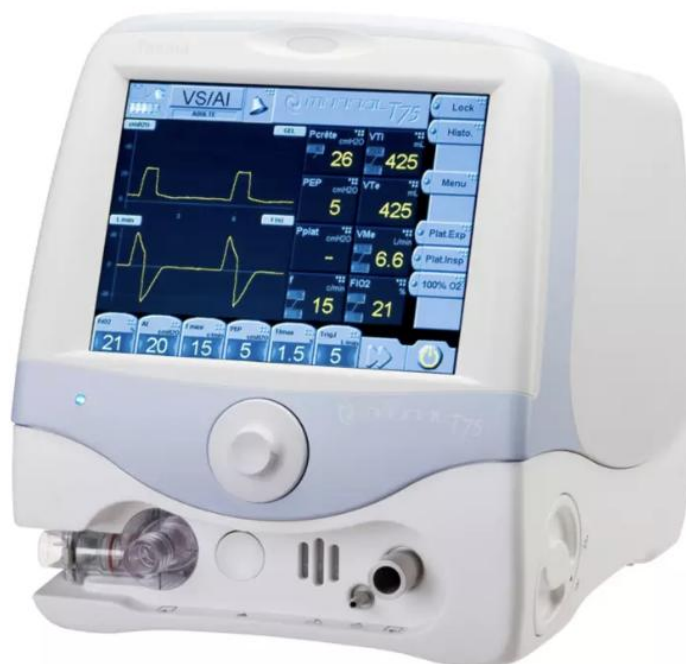
MONNAL T75 Mechanical Lung Ventilator
