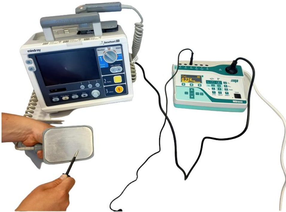
An example of measuring leakage current from the application parts using an alternative method
